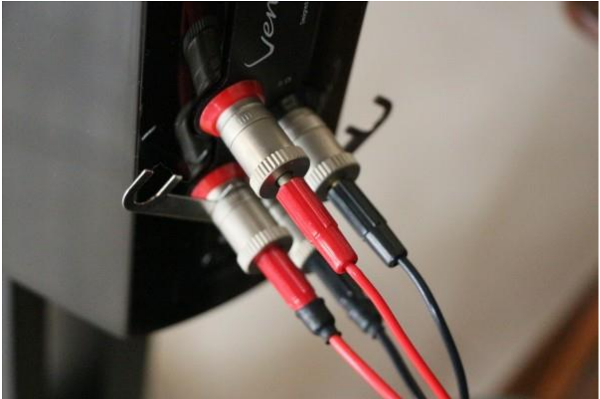
The speakers need to be bi-wired. Note the narrow rear of the speaker.
