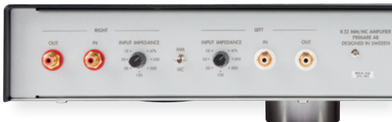
ABOVE: No XLR outputs, although the Teflon-insulated RCA sockets are top quality. Loading is selected via two rotary dials, denoting dual mono internals
