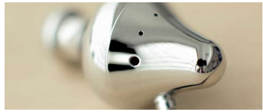
The differently sized vents on the rear of the housing are responsible for airing the interior. Thus the dynamic driver with its 16 millimetre diaphragm can move freely, since the air pressure is regulated inside.
