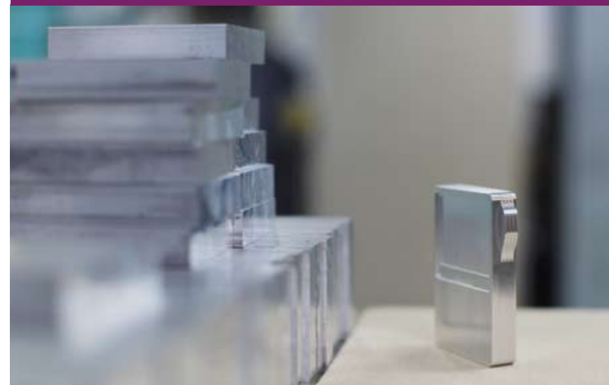
The Body of the AK-120 is machined from a solid aluminium billet on a CNC lathe. Though this process ensures absolute precision, each raw body is then painstakingly checked. At 13 precisely defined points, measurements are taken with an allowed tolerance of only 1/100 millimeter.
