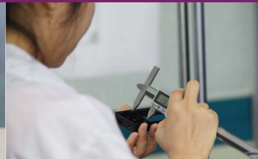
The Body of the AK-120 is machined from a solid aluminium billet on a CNC lathe. Though this process ensures absolute precision, each raw body is then painstakingly checked. At 13 precisely defined points, measurements are taken with an allowed tolerance of only 1/100 millimeter.
