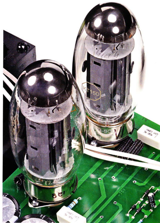
KT150 power output valves have very large anodes (grey) to dissipate heat, allowing them to handle high power.
