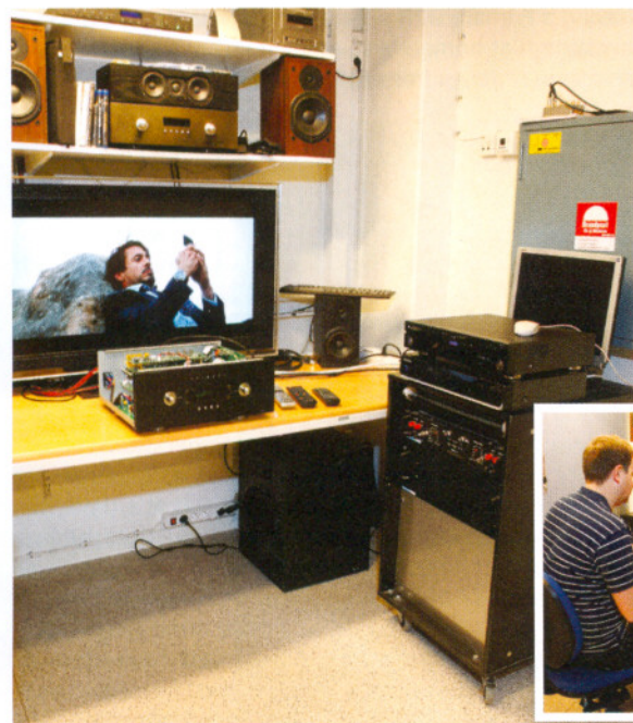
LEFT and BELOW: Checking one of the first SPA22 AV amplifiers, comparing it against Primare's references. Construction is modular, allowing for planned upgrade 'cards' to be slotted in
