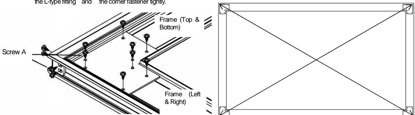
Set screws and slightly fix at all 4 corners temporarily first before tightening all screws.
