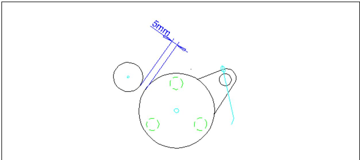
4. Fix the belt around the -platter and the motor-pully. The inner-platter has **one** separate groove, the motor-pully has **two** grooves:
