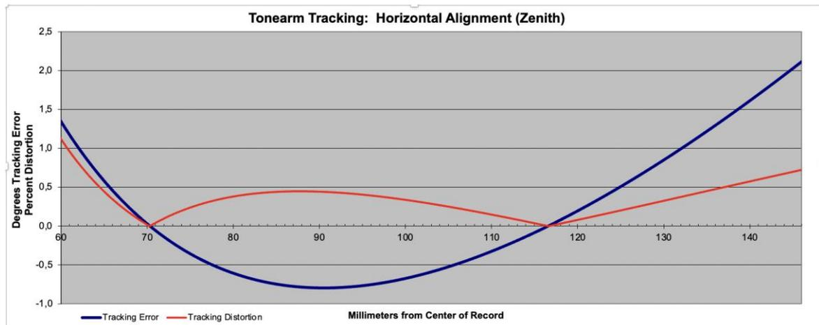
Here we can see the same condition as before, but the geometry is Löfgren B. Because the inner null point is shifted more from the centre, we got a more considerable tracking error at the end of the record and, with it, related distortion higher. But the integration of the distortion on the whole record will be lower than in the previous case.
