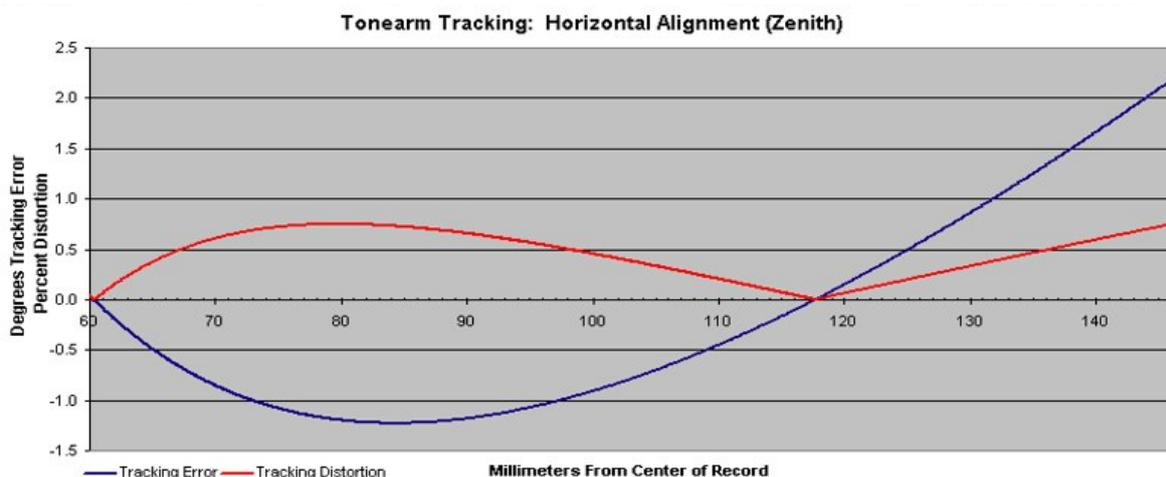
Compared to Baerwald or Lofgren B, you will get lower distortion at the very beginning and very end of the record, with the downside of higher distortion in the area between the null-points.
