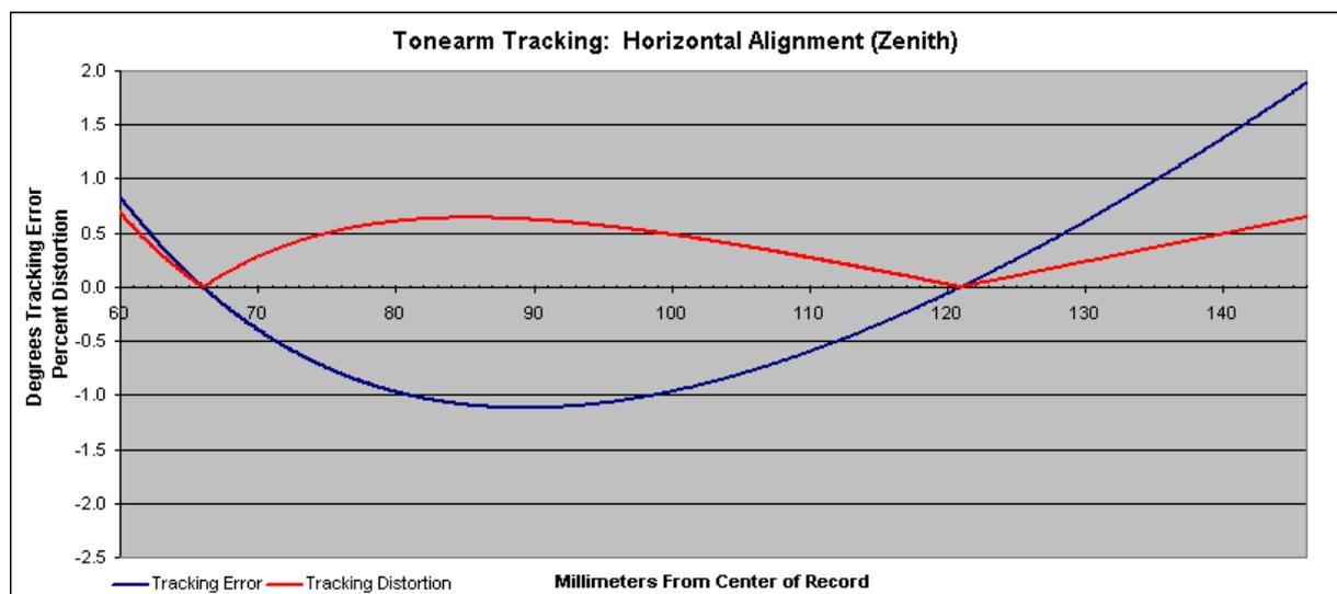
From the beginning, the tracking error has a positive value, but between null-points is negative and after the inner null-point positive. That is why our formula mentioned above counts with the absolute value of tracking error. The red curve represents distortion. The Baerwald geometry works universally and equally well for many musical tastes. An excellent allrounder, which is why it is so popular.
