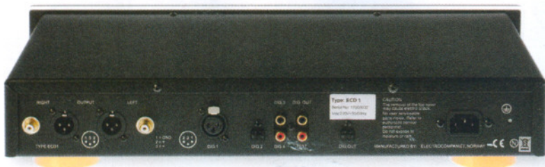
ABOVE: Plenty of connections on offer with one optical and two coaxial S/PDIF digital inputs joined by an AES/EBU (XLR) option. There are coaxial and optical digital outputs as well as both single-ended (RCA) and balanced (XLR) analogue outputs
