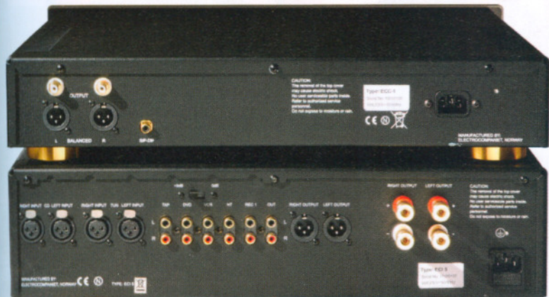
ABOVE: Single-ended and balanced (XLR) outputs on the CD player meet balanced inputs/preamp outputs on the amp, four line ins and a pair of 4mm speaker terminals
