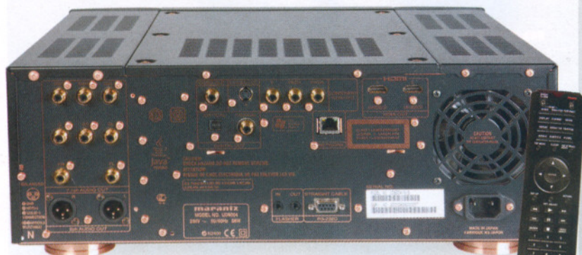
ABOVE: Balanced stereo XLRs are joined by 7.1 channel RCAs, an Ethernet connection for firmware updates and to access BD Profile 2.0 Bonus View content, plus two independent HDMI outputs (for audio and/or video)
