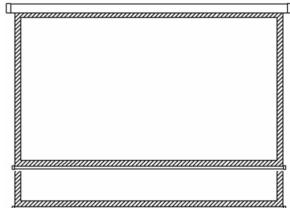
After adjustment, push the **UP** button of the IR remote controller. When the screen is rolled back approx. 20-30cm, push the **STOP** button.
