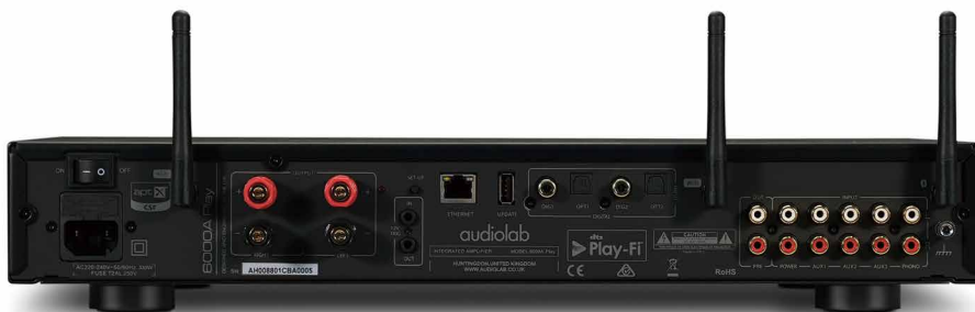
Around the back are three aerials for Wi-Fi and Bluetooth, plus a wide range of analogue and digital cable connections
