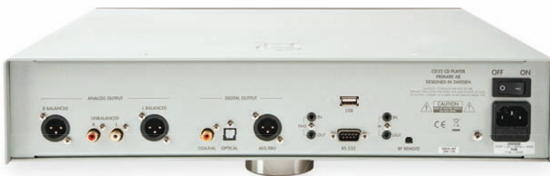
ABOVE: Outputs are single-ended and balanced, there are 3 digital outs, and RS232, IR and triggers are included too. USB input offers only MP3 and WMA file playback
