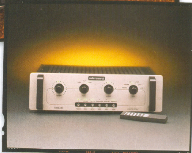
ABOVE: From 1996, the LS22 tube stereo line stage boasted remote control as a $500 extra RIGHT: The LS25 preamp from 1998 – inside were four 6922 twin triodes
